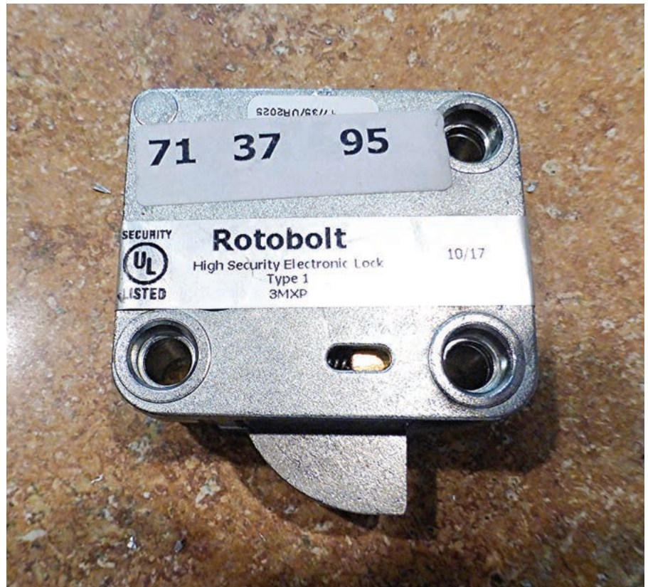
FIGURE 15. The code on the label is a service code that might be retained by the manufacturer. Since the author's customer received a new keypad from Cannon, the author assumes Cannon does not keep records of service codes — or they only use the service code when they send out a tech for a warranty issue.
