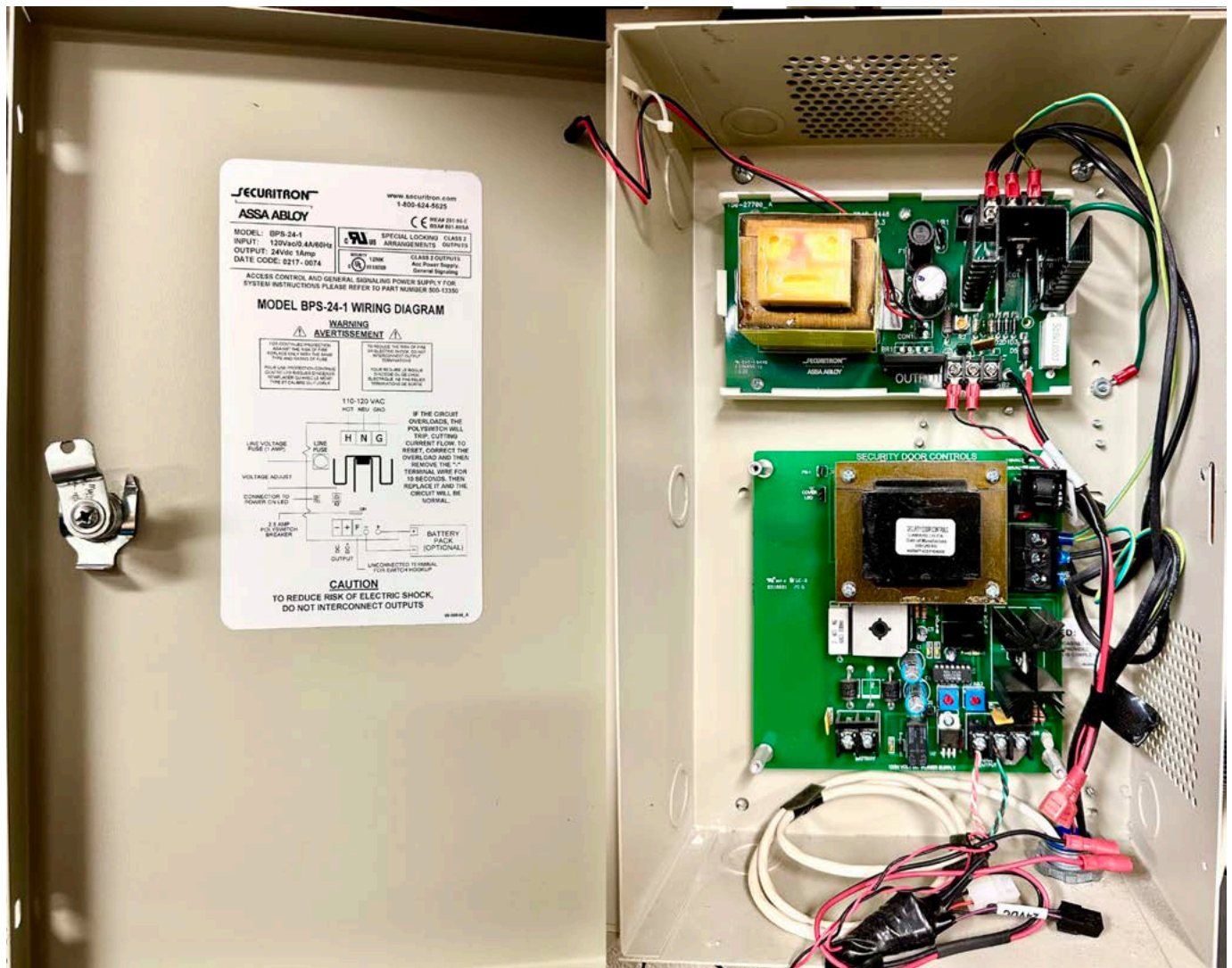
FIGURE 3. Here is a picture of a UL Listed Securitron power supply with two different power supply boards mounted in it. This would never meet UL. Fortunately, this is just a bench testing setup at the author's shop.
