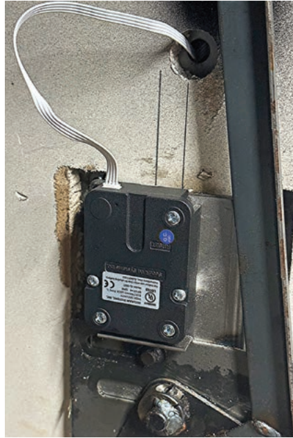
FIGURE 13. The author installed a SecuRam Basic swing bolt. Notice there is no reload trigger plate or external reload on this safe.
