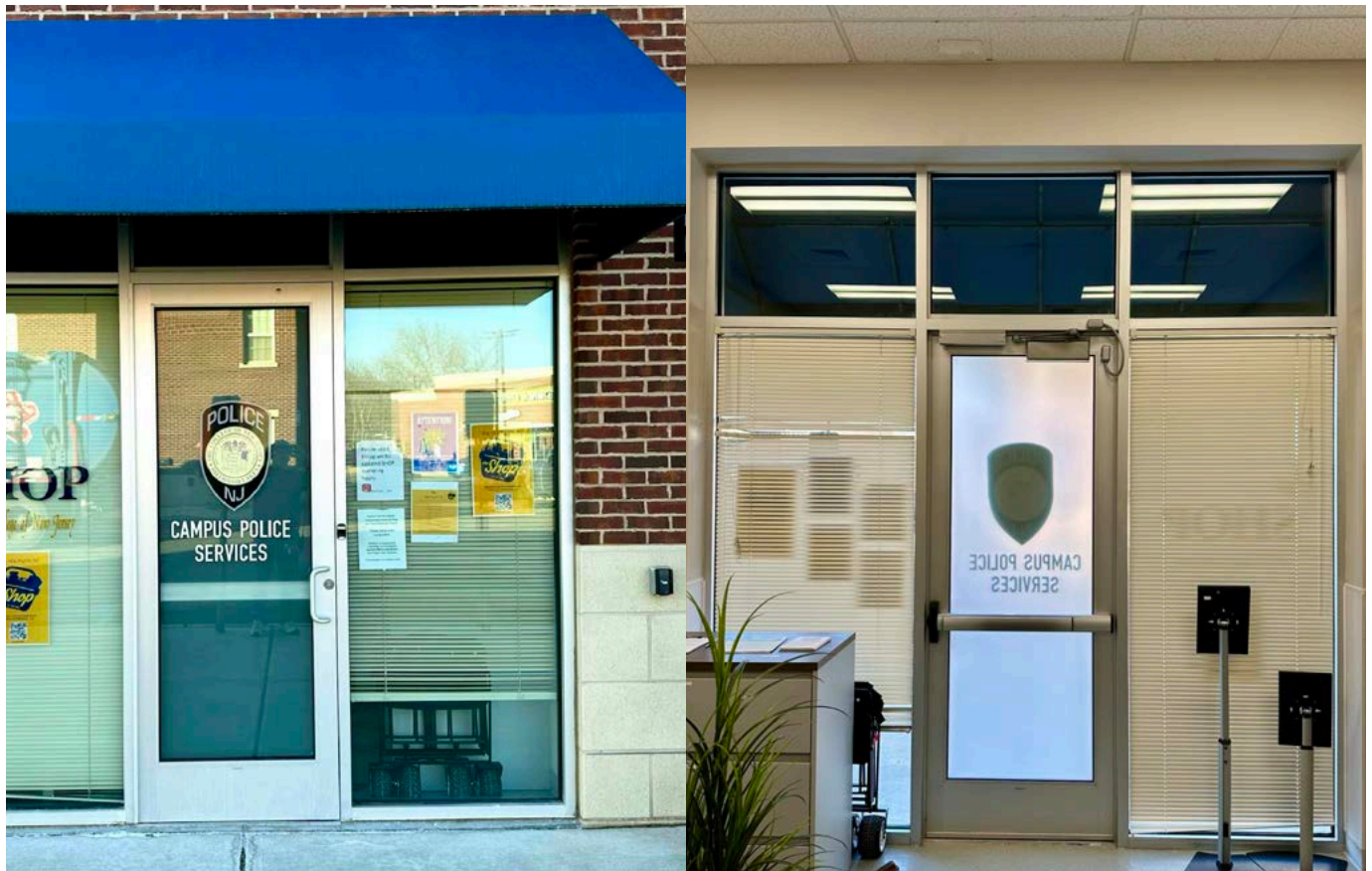
FIGURE 7. This is an example of a door that would be UL294 certified, as both the ingress and the egress side of the same door are controlled. (TCNJ Campus Police Sub-Station)
