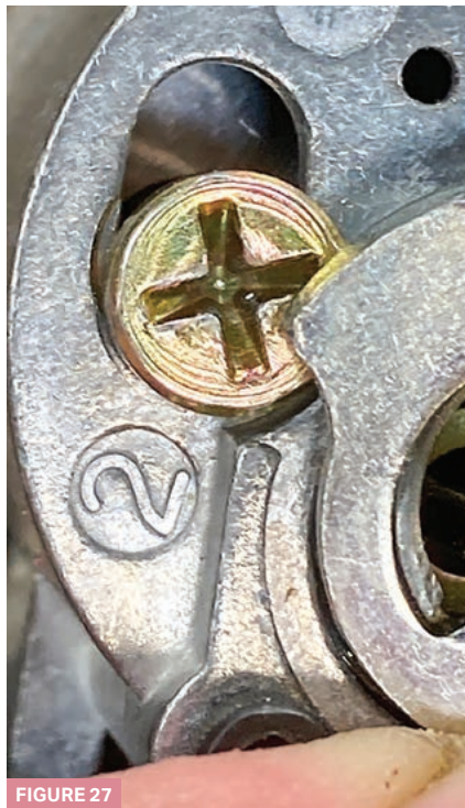
FIGURES 27 AND 28. The head of the rim cylinder screw is catching under the cam because the cam is not pointing down.
