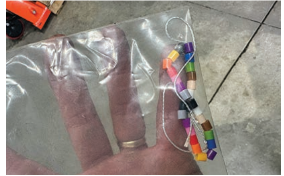
FIGURE 4. This string of beads with lead shot on one end was made for finding the mini lock inside of a safe. It was purchased at SAFETECH 2019 from Taylor Technologies.
