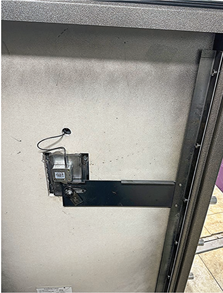
FIGURE 3. This photo was from a previous lock replacement job. The lock is very close to the BCH as it blocks the carrier bar from moving.
