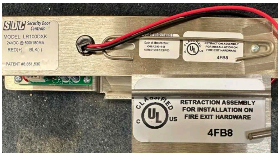
FIGURE 8. This is an example of an electric latch retraction add-on device. This is used to electrify an existing exit device that is not currently controlled and saves on the cost of a completely new device.
