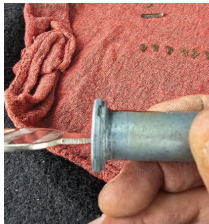
FIGURE 27. Here, you can see the sidebar down completely. This depth is correct. Now place a mark on the HPC machine to reference it.
