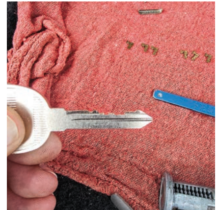
FIGURE 34. The author now has a key where he can replicate the cuts over and over because he's using the plastic screen of the HPC machine just like an HPC card.
