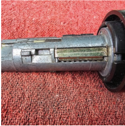
FIGURE 2. This is an example of the GM 10 cut (B102) type. Here, we see the sidebar extended and the spring cap. Be careful not to break the legs of the spring cap.
