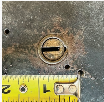
FIGURE 8. The author drilled for the fence at \frac{5}{8} " up.
