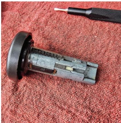
FIGURE 5. The spring cap is almost completely out at this point. From here, the author feels confident about getting it off without breaking it.
