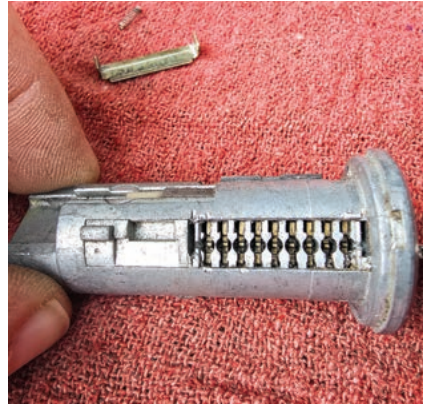
FIGURE 9. The author has stuck a key blank into the lock, which causes all of the wafers to raise as much as possible. In this photo, you can see the wafers in their individual chambers.
