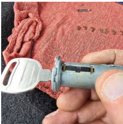
FIGURE 26. All that is required is to place only that wafer in the lock and start cutting little by little until the sidebar stays completely collapsed.
