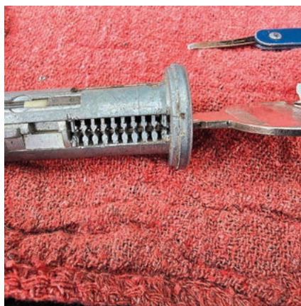
FIGURE 15. The key blank is inserted in the lock, and you can see the marking tool the author will be using to make marks on the key blade.
