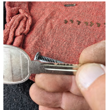
FIGURE 28. Here are the correct depths for the first and second spaces. Now we have 1 and 2; we just need 3 and 4
