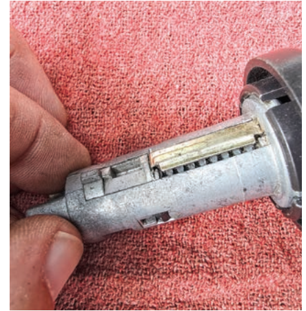
FIGURE 4. It helps to lift the spring cap from both sides. This will help release both legs at the same time.
