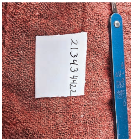
FIGURE 14. Here are the numbers from the wafers. These are the cut depths to use when starting to cut the key.
