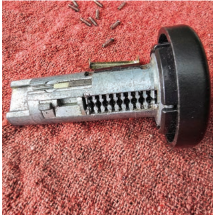
FIGURE 8. All springs are out of the lock, and the next thing to do is to start extracting wafers. Use a key blank to make this job quite a bit easier.
