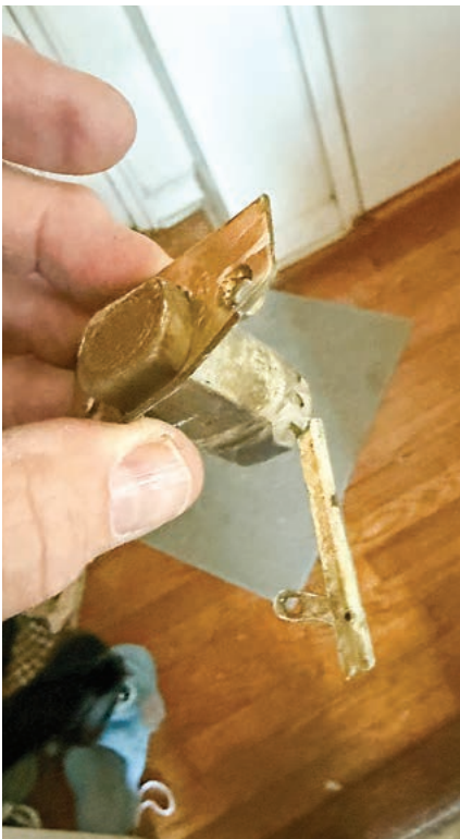
FIGURE 10. Here are the remains of an Arrow deadbolt that was ripped out of the door.
