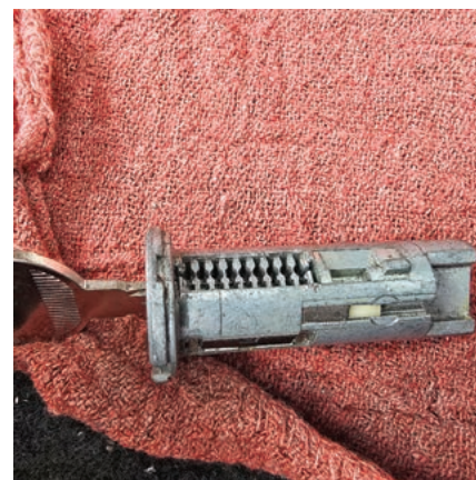
FIGURE 16. Notice the orientation of the key in this image. It is important to mark the key closest to you so you can see the marks when setting up the HPC machine.
