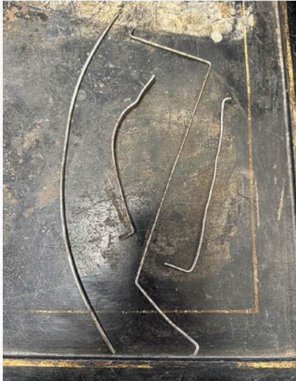
FIGURE 5. These are the author's homemade picking tools.
