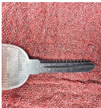
FIGURE 17. The author has made a mark on the key using each of the nine chambers. They are fairly uniform in spacing.
