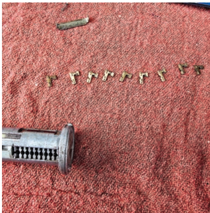
FIGURE 11. At this point, the author has the lock completely disassembled and has the wafers in order. Keeping them in order is very important.
