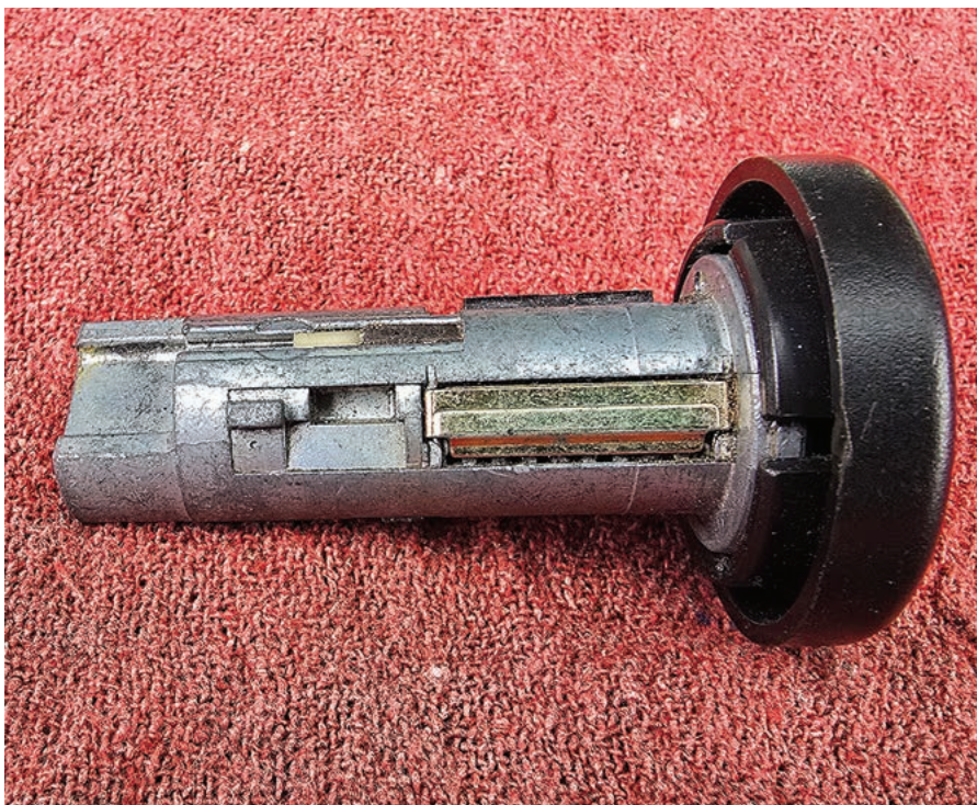
FIGURE 1. Begin by getting the lock to the work area. In this case, a little sidebar manipulation was required. This is the GM 10 cut (B102) type.
