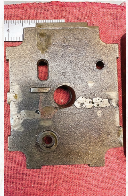
FIGURE 22. The lock cover has been repaired.
