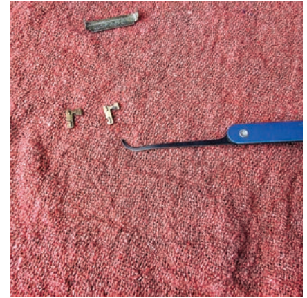
FIGURE 10. Often, using a key blank will not cause the wafers to raise enough. In that case, a large hook pick like the one here is exactly right for the job.
