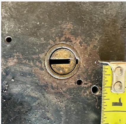
FIGURE 7. The author drilled for the fence at \frac{1}{2} " right.
