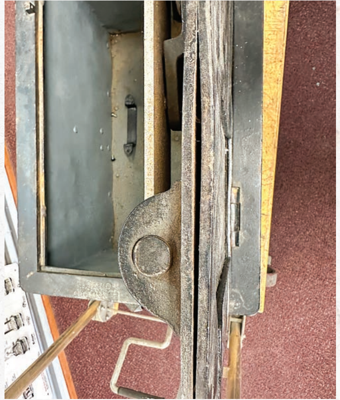
FIGURE 17. The door is double-plated.
