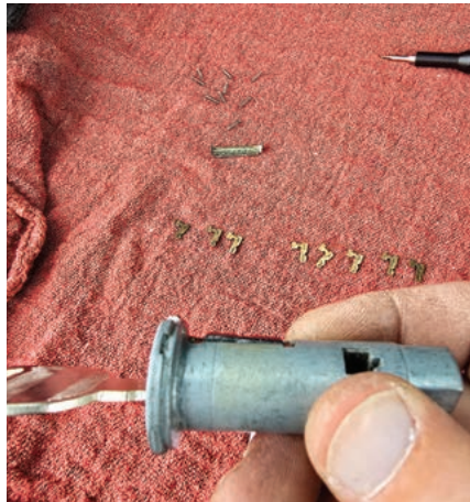
FIGURE 32. This is what it will look like if you do not have the depth set correctly. The sidebar here is quite high, and the lock will not turn.
