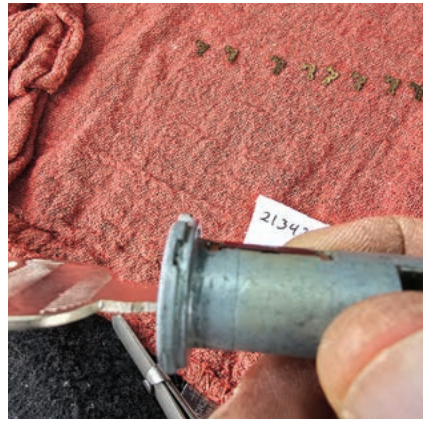
FIGURE 30. Each time the author determines a new depth, he verifies the sidebar is completely collapsed. As long as it is, he places a mark on the machine.
