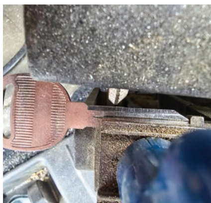
FIGURE 18. Now take the key to the HPC machine and line up each mark you made with the broken pick. As you line up each mark with the center of the cutting wheel, make a mark on the plastic of the machine.
