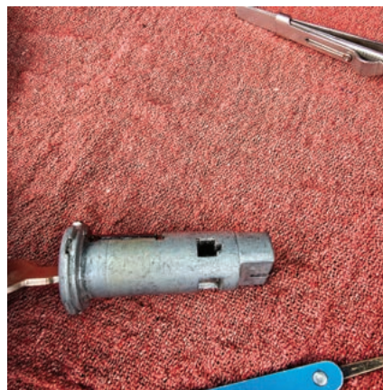
FIGURE 36. Here, you can see that the author has successfully cut a key using the markings on the HPC machine. This side is the same side he used to mark out the spaces on the key.
