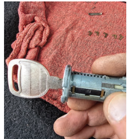
FIGURE 25. Since there is a 2 depth in the first chamber of the lock, do that one next.
