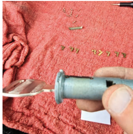
FIGURE 33. Here is when the author found the fourth and last depth. He marked it on his machine and now has a full setup for cutting the keys.
