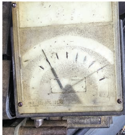
FIGURE 24. Here is where the 1 depth mark will be. This is the depth that the cutting wheel just touches on the edge of the key blade.
