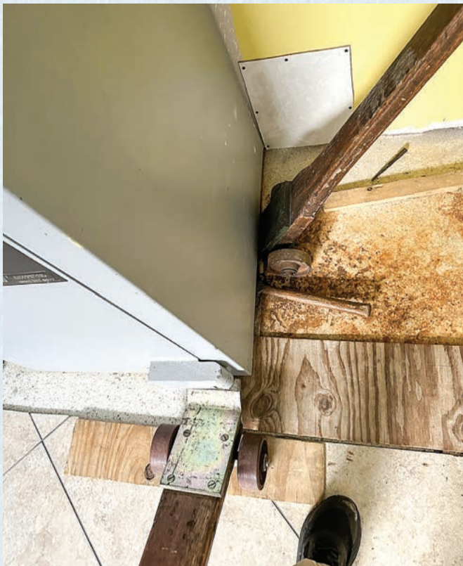
FIGURE 9. On the second job, two Johnson bars were needed just to break the safe free.
