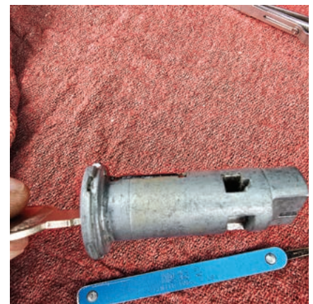
FIGURE 37. The author has turned the key over and cut the other side using only the marks on the HPC machine. As you can see from this picture, the cuts match, and the key is finished.
