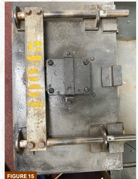
FIGURES 14 AND 15. The boltwork is in the unlocked position in Figure 14 and locked in Figure 15.
