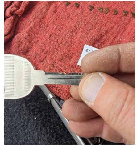
FIGURE 31. Here, the author has cut the third depth and marked the machine.
