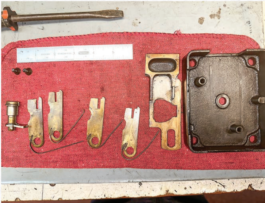
FIGURE 25. Here is an exploded view of the lock.
