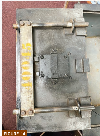
FIGURES 14 AND 15. The boltwork is in the unlocked position in Figure 14 and locked in Figure 15.
