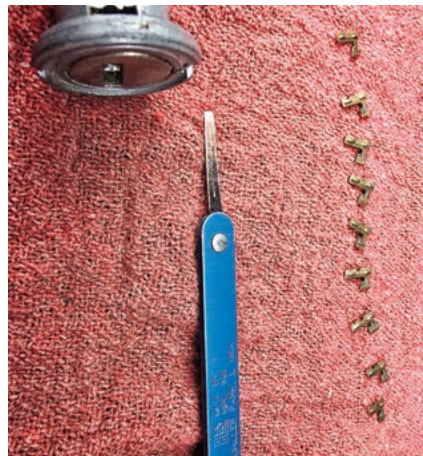
FIGURE 12. The wafers are laid out in the same order they came out of the lock, and the author will be marking the key with a broken pick.
