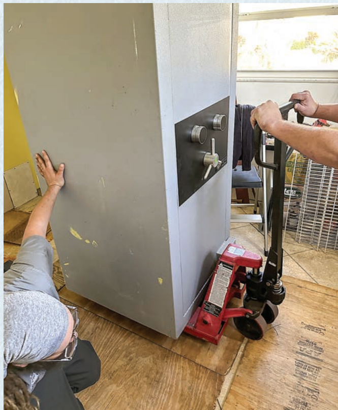
FIGURE 13. Here, the front wheel is stuck in a seam of plywood that is protecting the flooring.
