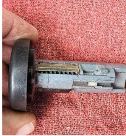
FIGURE 3. In this picture, the author has started slowly removing the spring cap. Notice he is not lifting either side too much.
