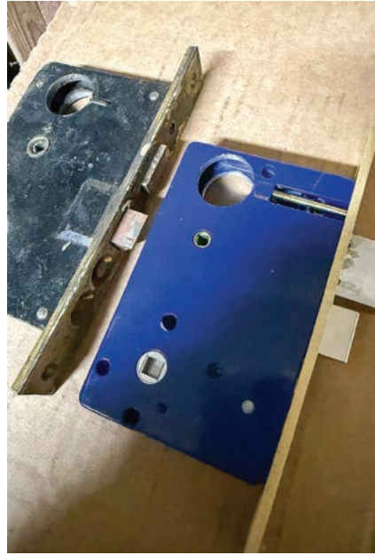
FIGURE 18. The new mortise lock's deadbolts are significantly larger than the old ones.
