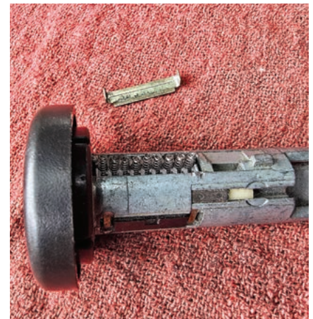
FIGURE 7. The spring cap is completely removed, and all springs are exposed. The next step is to remove all of the springs.
