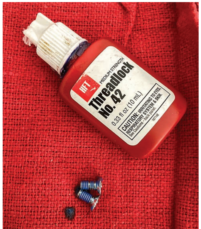
FIGURE 17. The author put a bit of threadlock on the screws before attaching them.
