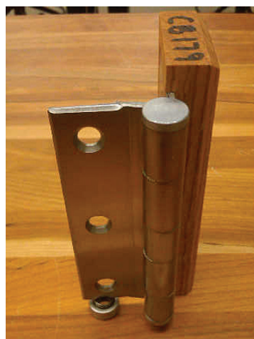
Figure 6. This image shows a half mortise hinge as it would appear on the pull side of a closed door.
