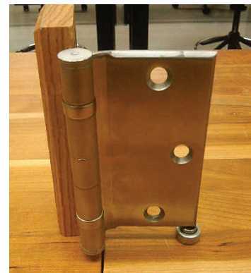
Figure 5. This half surface ball bearing hinge is as it would appear on the pull side of a closed door. The wooden block slightly to the left of the knuckle represents the frame.
