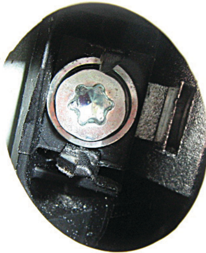
Figure 1. Some vehicles have a screw in the door edge (under a grommet) that you can loosen; you can then remove the door lock cylinder.
