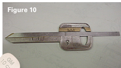
Figure 8. Using a scope like this one with a wafer depressor attached, you can move the wafers and read the depths directly.
