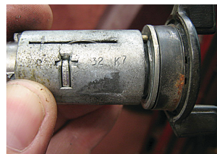
Figure 4. You also can look for a code on the ignition cylinder. Once the cylinder is out, you'll find the code stamped in the side of the housing.
