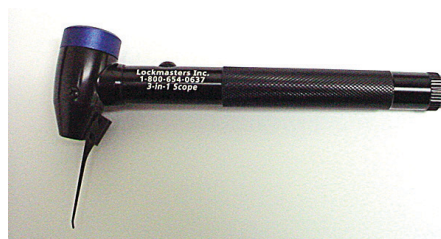
Figure 8. Using a scope like this one with a wafer depressor attached, you can move the wafers and read the depths directly.
