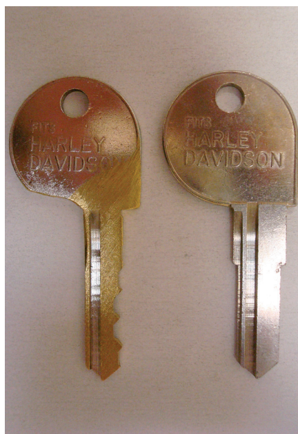
Figures 5 and 6. These images show an original X133, and the modified version to fit into a U-Change cylinder.
