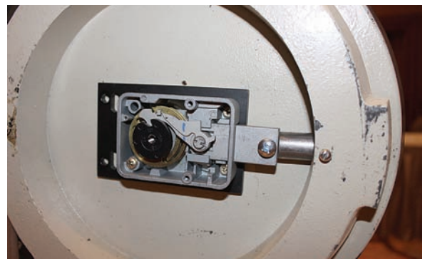
Here is the finished Mosler retrofit.
