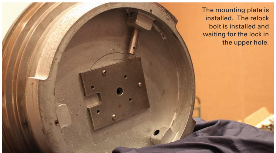
Shown here is a similar Diebold Lug door with the 180-55 lock, as used in the class.
