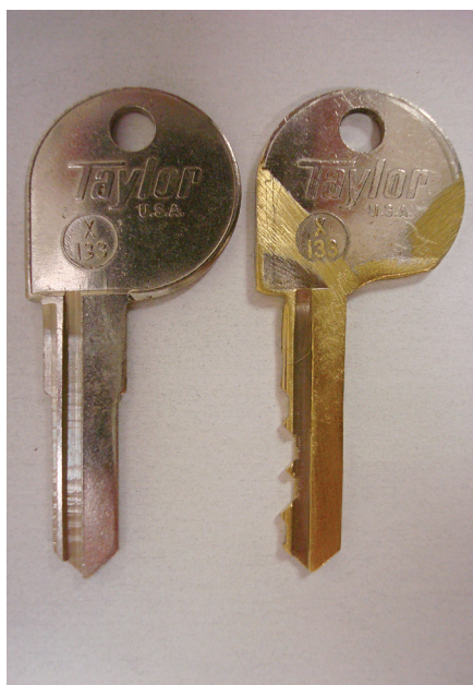
Figures 5 and 6. These images show an original X133, and the modified version to fit into a U-Change cylinder.
