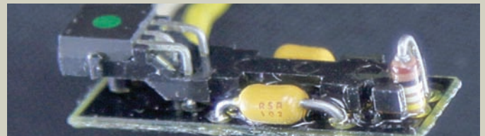
Figure 5. Shown here is a Passlock I circuit board with one sensor (marked with a green dot) and one resistor.
