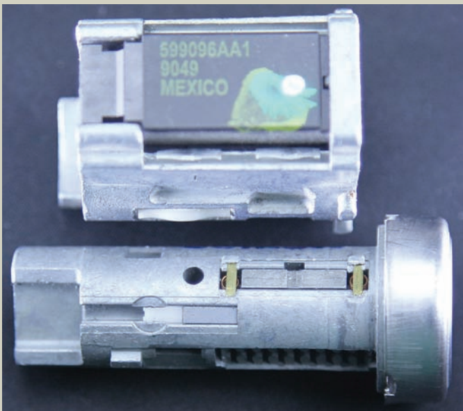
Figure 1. When the driver attempts to start the car, a magnet contained in the lock plug passes by a Hall Effect sensor.
