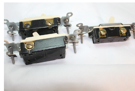
Figure 9. The switch on the right is a standard on/off wall switch for your house. Notice that the two terminals are the same brass color. The two on the left are three-way switches. Also notice the single black terminal, which is the common terminal, and the two brass terminals, which are connected together to create allow the two switches to control the same light.
