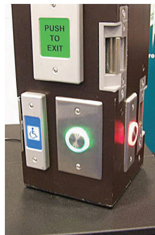
Figures 7 and 8. This is just a sampling of the variety of switches available for locksmiths to use for electronic access control.
