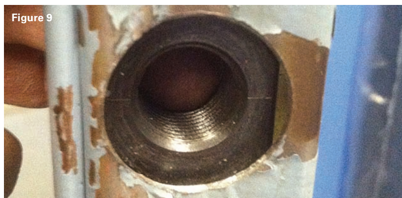
Figure 9. The die is properly inserted. If you put it in wrong, the threaded hole in the die won't be centered.
