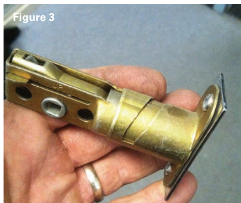
Figure 3. The icing on the cake: an adjustable Kwikset deadbolt. He could've made it 2¾" if he'd known to do it. I wouldn't have installed the way he did, but at least the backset would've been right.
