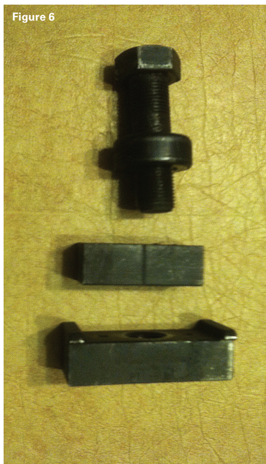
Figure 6. This image shows the parts of the Pit Bull (see "Working Without a Mortise," p. 39). From top to bottom: the large bolt that tightens the tool on the door, with a thrust bearing on it; and the exterior and interior parts of the die that forms the mortise.
