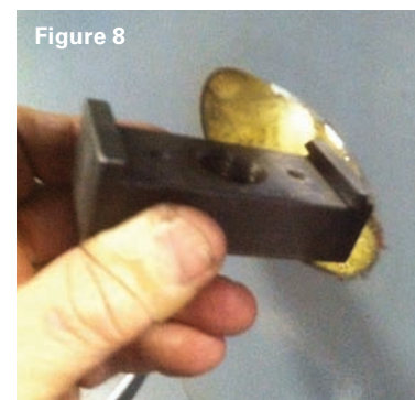
Figure 8. The inside die is inserted in the door. The two large tabs on one side of it face away from the door's rolled edge seam. Be careful not to drop it inside the door or you'll weep bitter tears.
