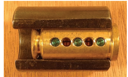
Figure 4. When you feel confident about your skills, disassemble the cylinder again and add another pin to the first chamber.
