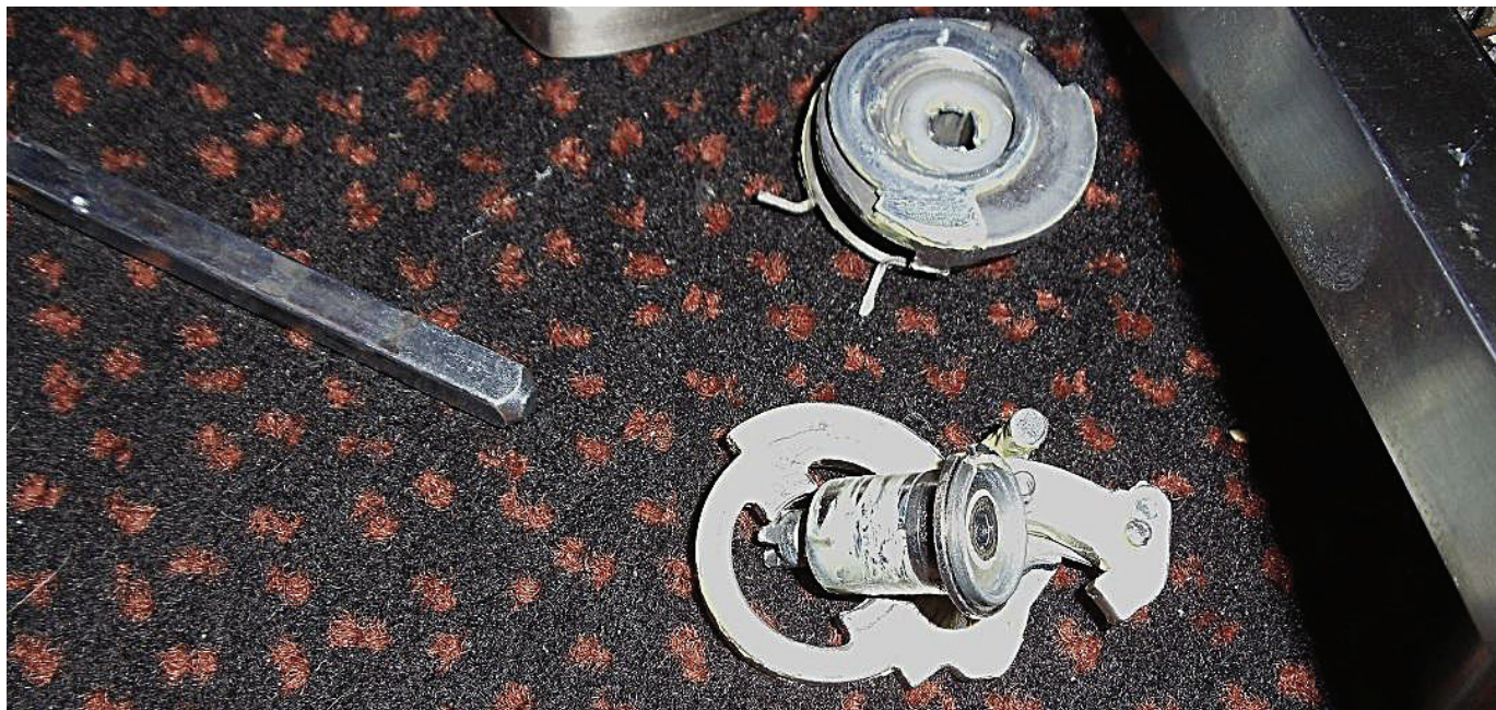
Figure 6. This image shows the clutching assembly's parts: a return spring, a pressure plate and the handle spindle.
