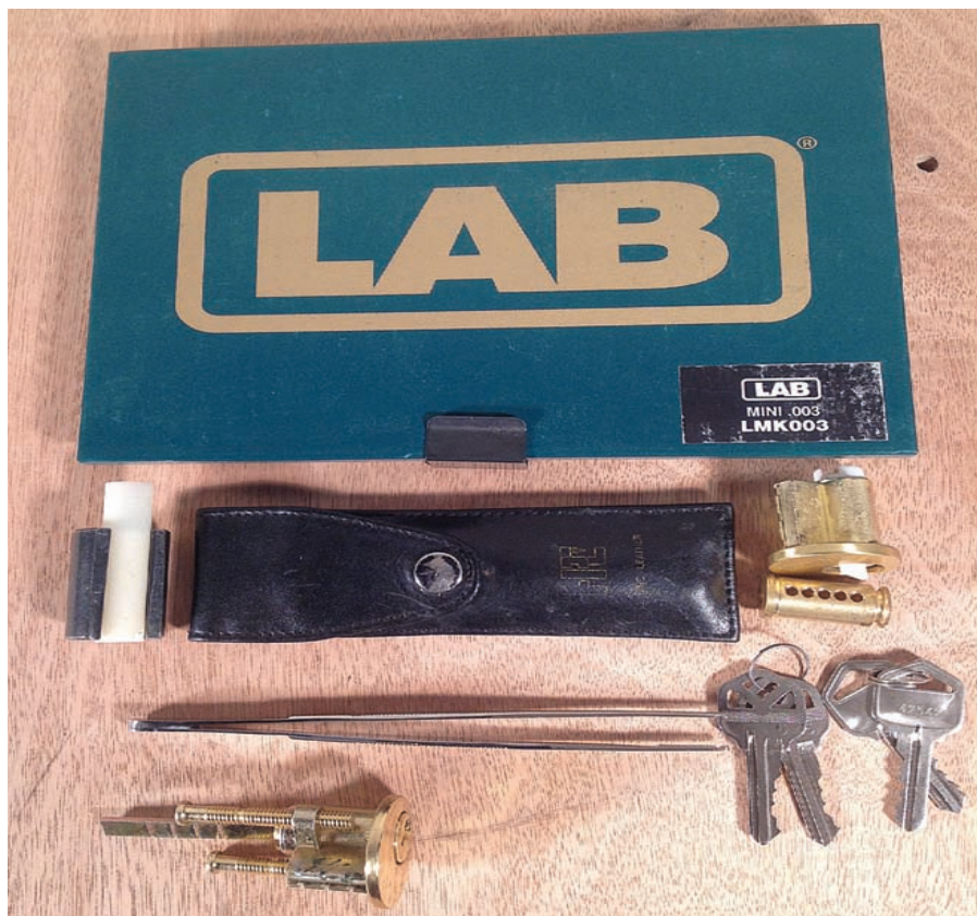
Figure 1. You'll need a basic lock-pick set, a pin kit and pinning equipment (especially tweezers), and several pin tumbler cylinders from different manufacturers.
