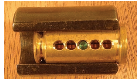
Figure 3. Take any random pin, and re-pin the cylinder in the third chamber only.
