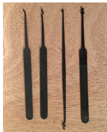
Figure 2. Common picks include (from the left) a hook or "feeler" pick, a rake, a half-diamond and a ball pick.
