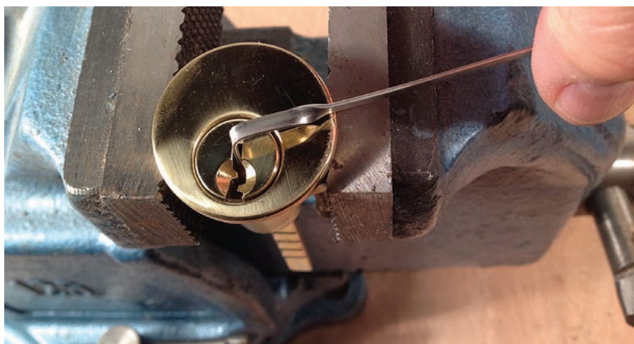
Figures 5 and 6. In the top image, the wrench is positioned to turn left. In the bottom image, the wrench is on the other side of the cylinder, but it's still positioned to turn left.
