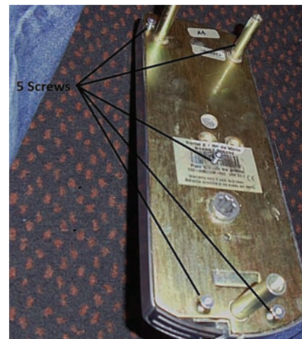
Figure 2. Remove these five screws to take off the back plate.
