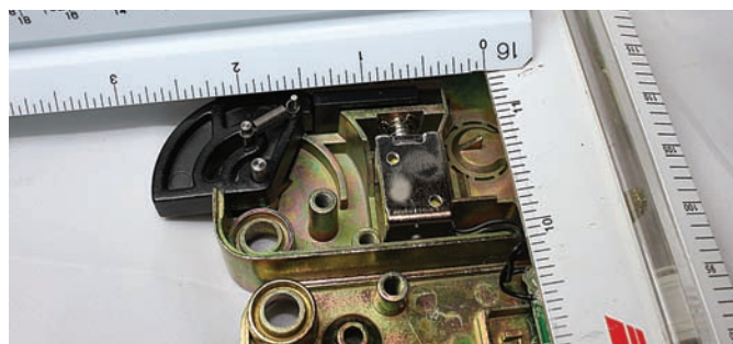
The rulers are little deceiving in the picture, but the top ruler is sitting on the \frac{1}{4} " mark above the 11" mark that's centered over the center of where the spindle on a mechanical lock is located. The solenoid is about \frac{11}{16} " from the spindle hole center; take your pick of where to drill to take out the slide between the solenoid and the swingbolt. Taking out the slide requires drilling all the way through the slide. An alternative location or method is to drill carefully through the lock case at the "C" clip on the solenoid and move it back.
