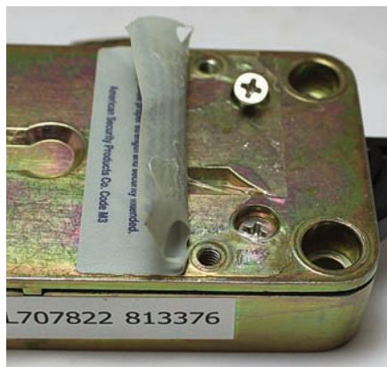
The label hides a couple of screws that keep the case together.
