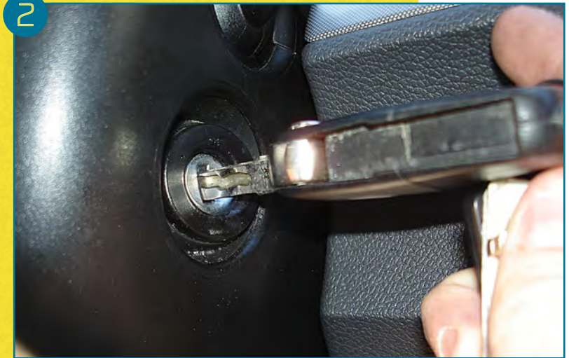
Figure 1. Removing the top shroud screw. Figure 2. Turning the ignition cylinder with the key. Figure 3. The top shroud lifts for easier access. One of the two screws holding the lower shroud is shown. Figure 4. Removing the lower shroud. Figure 5. A working key allows for removal of ignition cylinder.
