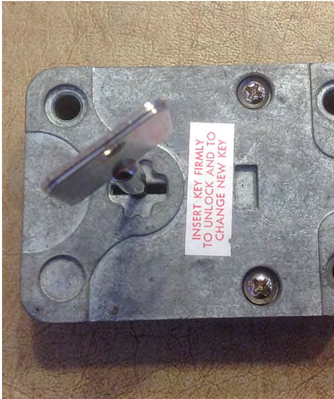
Figure 2. The key stops at about the 2 o'clock position
