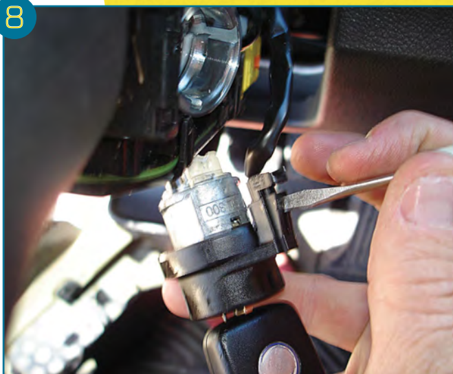
Figure 7. Removing the cylinder from the housing. With the skewer in place and the key turned on, you can push in to depress the retainer and remove the cylinder.
