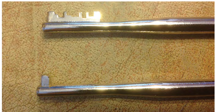
Figure 11. A key that has been filed off, leaving only the very tip.
