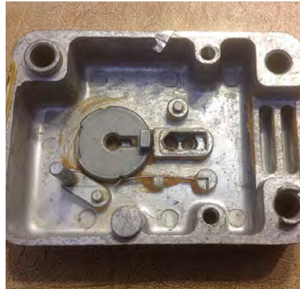
Figure 9. Lock with bolt removed to show the cam that rotates to pull back the bolt.
