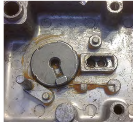
Figure 10. Here's the position the cam might be in if the spring is broken.
