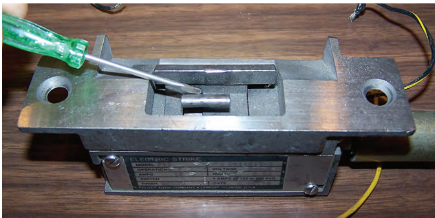
This is an example of a strike with a latch-bolt position monitor switch. The monitor switch is moved with a screwdriver to simulate a latch bolt in the keeper.
