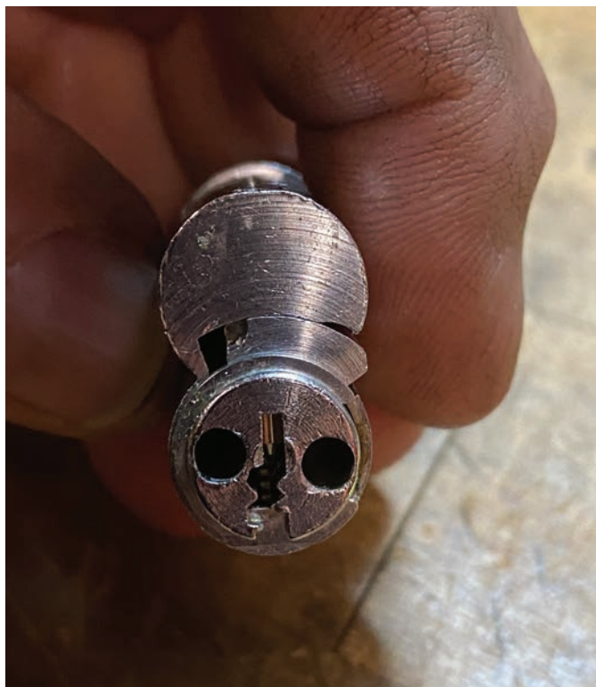
Figure 21. Combine the core as seen here, where both the plug and the dog are in the locked position.
