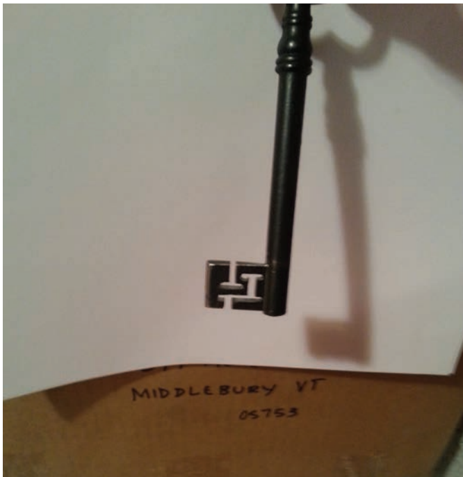
Figure 6. Next, I finished up the wards with a very thin file using the smoke-and-file method, only I used a black Sharpie pen, which doesn't rub off as easily as smoke. I inserted the key as if impressing and filed where necessary. Being persistent, I got a working key.
