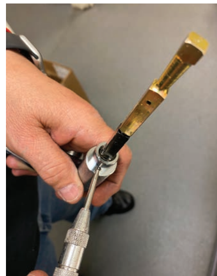
Figure 14. The author is using an automatic center punch to seat the pin.
