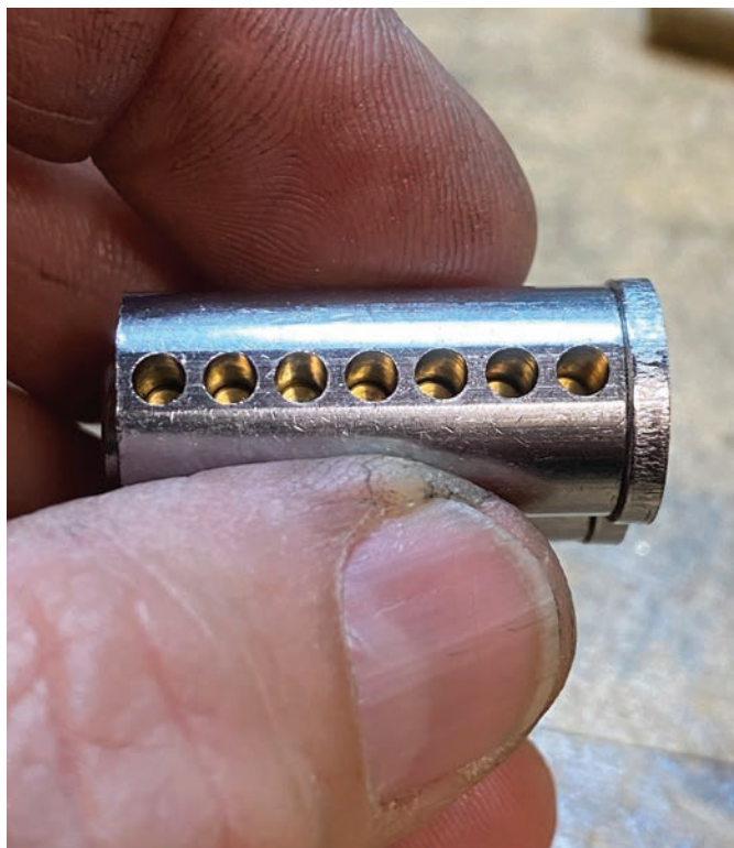
Figure 22. When you tilt the core, all the pin stacks are the same height.
