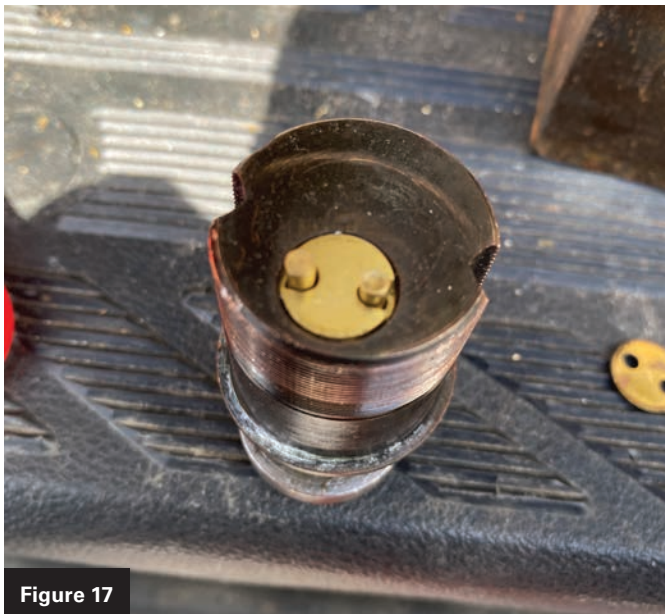
Figures 15-18. These images show the sequence of assembling the parts when changing a cam on a BEST mortise cylinder.
