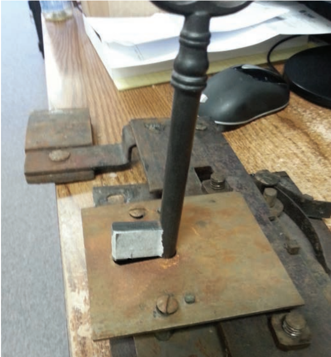
Figure 4. The key was filed flat and cut to fit the lock opening. Putting tape on the key blade allowed me to mark the wards I would need to cut into the key blade, which would allow the key to operate the lock.
