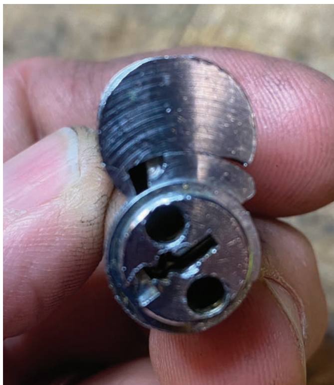
Figure 19. On the back of the core, the plug is turned, but the locking dog is in the locked position.
