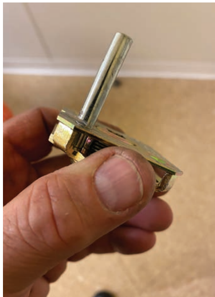
Figure 3. On the outside spring cage of a 45H, one of the studs is cut off, and the second one is partially cut.
