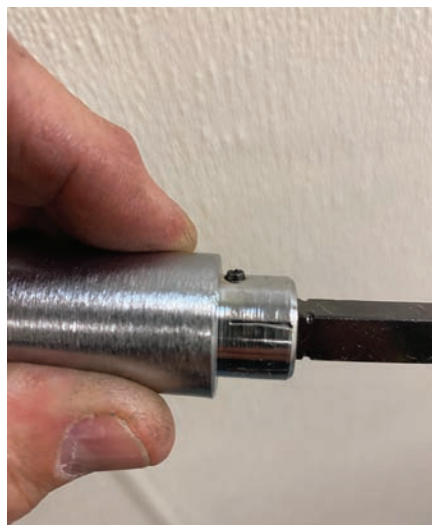
Figure 13. Sometimes the roll pin on the outside lever of a 45H lock is projecting out of its hole a bit.
