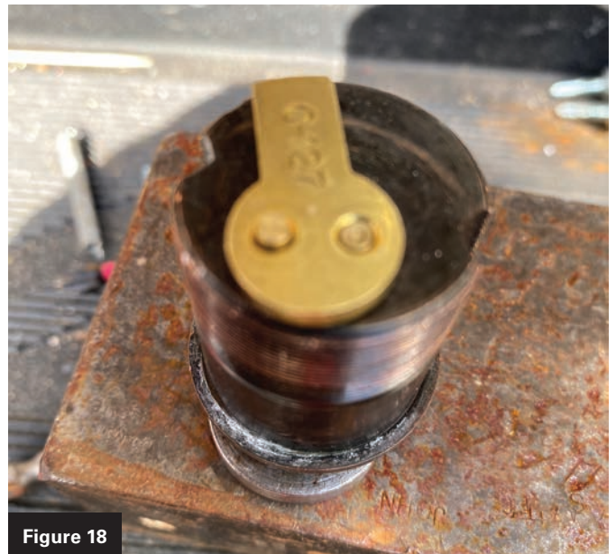
Figures 15-18. These images show the sequence of assembling the parts when changing a cam on a BEST mortise cylinder.
