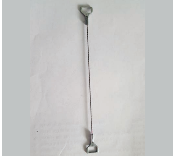
Figure 5. Intersecting points marked on the key blade were where I needed to drill holes so I could cut or file the wards as needed. I found a small, round metal-cutting saw blade on the internet that let me cut the wards. The saw blade was spiraled and very sharp. It allowed me to take one end bracket off so I could place the saw blade into the hole drilled at intersecting points in the key blade and then replace the bracket. With the saw blade in place, I was able cut horizontal and vertical wards in the key blade.
