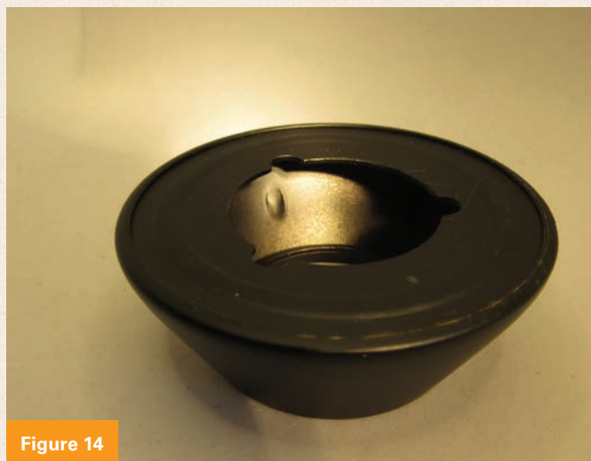
Figures 13 and 14. The collar is seen from two slightly different angles under different lighting, highlighting that the collar is completely hollow.
