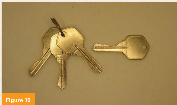
Figures 15 and 16. The keys are lightweight brass, and the shape is in the Kwikset “house bow” style.
