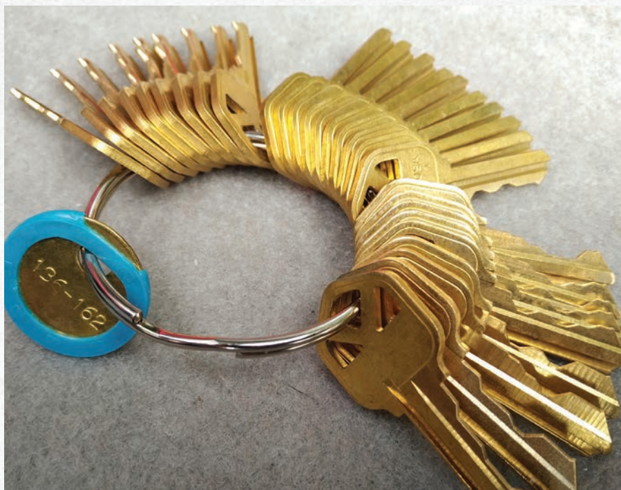
Figure 4. In this photo, the keys with a “1” final cut are in the foreground, while the middle section groups “3” final-cut keys (facing down) and the “5” final-cut keys are in the background.
