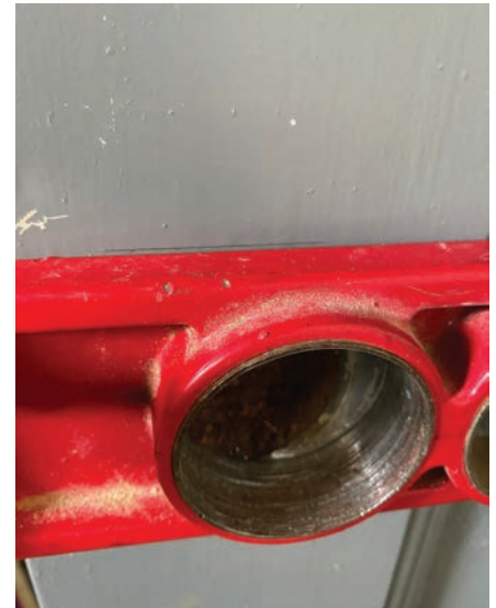
Figure 11. The author draws a line as a reference so he will know if the jig moves.
