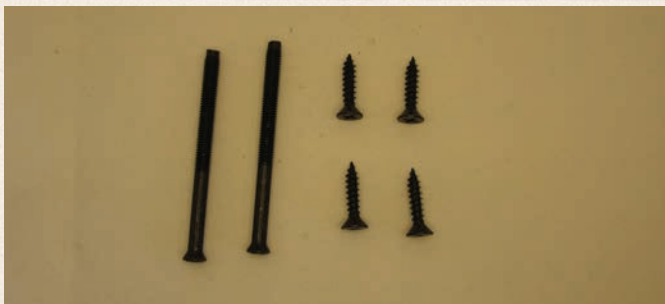
Figure 11. The deadbolt screw pack does not show impressive security.
