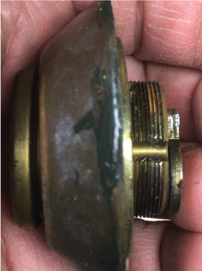
Figure 10. The customer's Lori deadbolt lock did not have a tailpiece but instead had a mortise cylinder with an Adams Rite-style cam.
