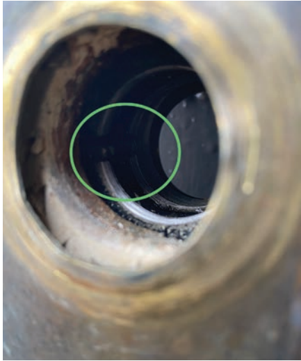
Figure 21. The green circle is around what holds the cylinder in place.
