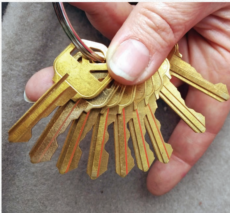
Figure 5. In the above example, the winning key is the second one from the right: 13531.
