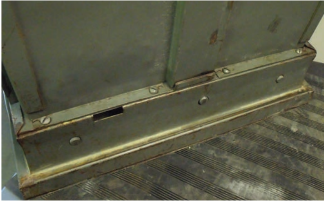
Figure 3. The first step was to remove the screws at the bottom and sometimes on the top edge.
