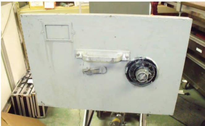
Figure 5. The many coats of thick paint made closing the doors very difficult.
