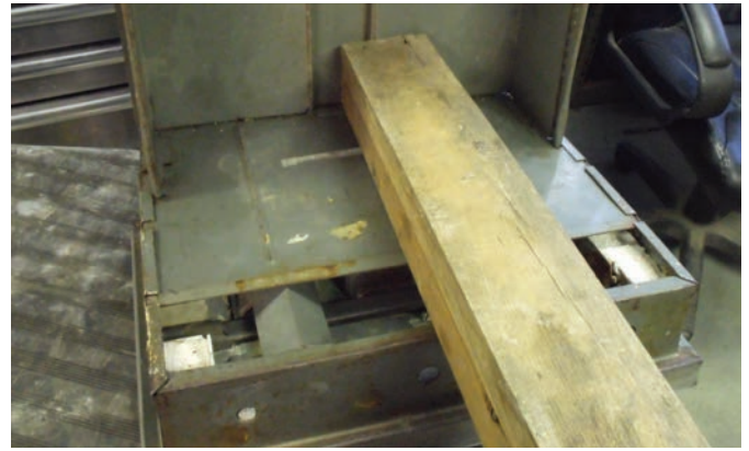
Figure 4. The author used a 4x4 to slam at bottom center to get it started.
