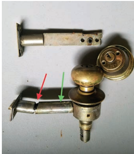
Figure 3. The green arrow points to the “extension” used to build a 5" latch. The red arrow points to where it connects to the 2 \frac{3}{8} " latch.
