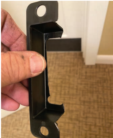
Figure 24. This is one of the black plastic dust boxes that come with each 45H lock (or what's left of it).
