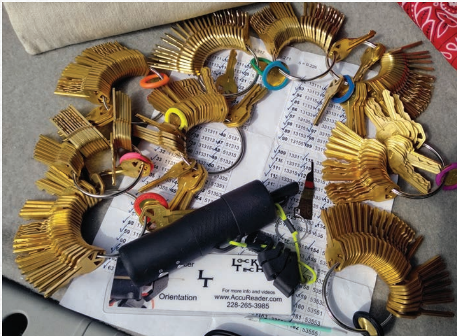
Figure 1. My all-in-one kit includes a LockTech decoder, lens cleaner and charger, plus nine rings of tryout keys and a key chart.
