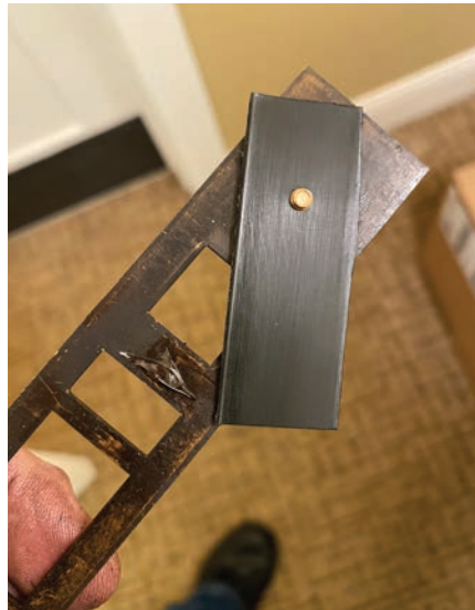
Figure 25. The author cut out a flat piece of the plastic dust box and trimmed it.
