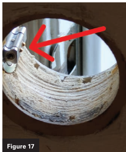
Figures 17 and 18. The bolt has contacts on it ( Figure 17 ) that will line up with the contacts on the motor once it's installed ( Figure 18 ).
