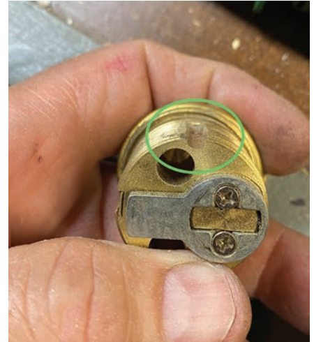
Figure 23. The author had to deepen the channel on the thumbturn so that it was about as deep as the BEST cylinder.
