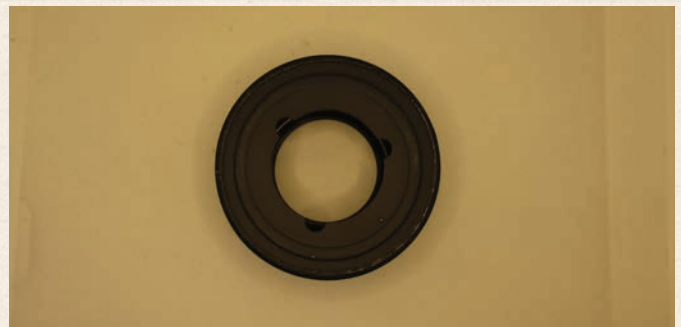
Figure 12. The deadbolt collar is made from steel but isn't hefty.
