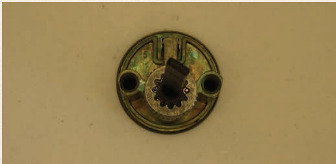
Figure 9. The back of the deadbolt is depicted without the collar.
