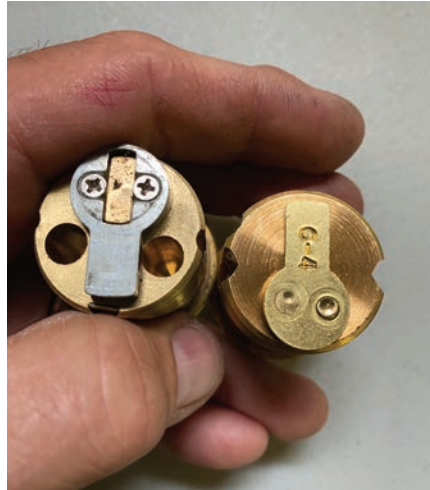
Figure 22. BEST mortise cylinders (right) have a deeper channel for the yoke to lock into.
