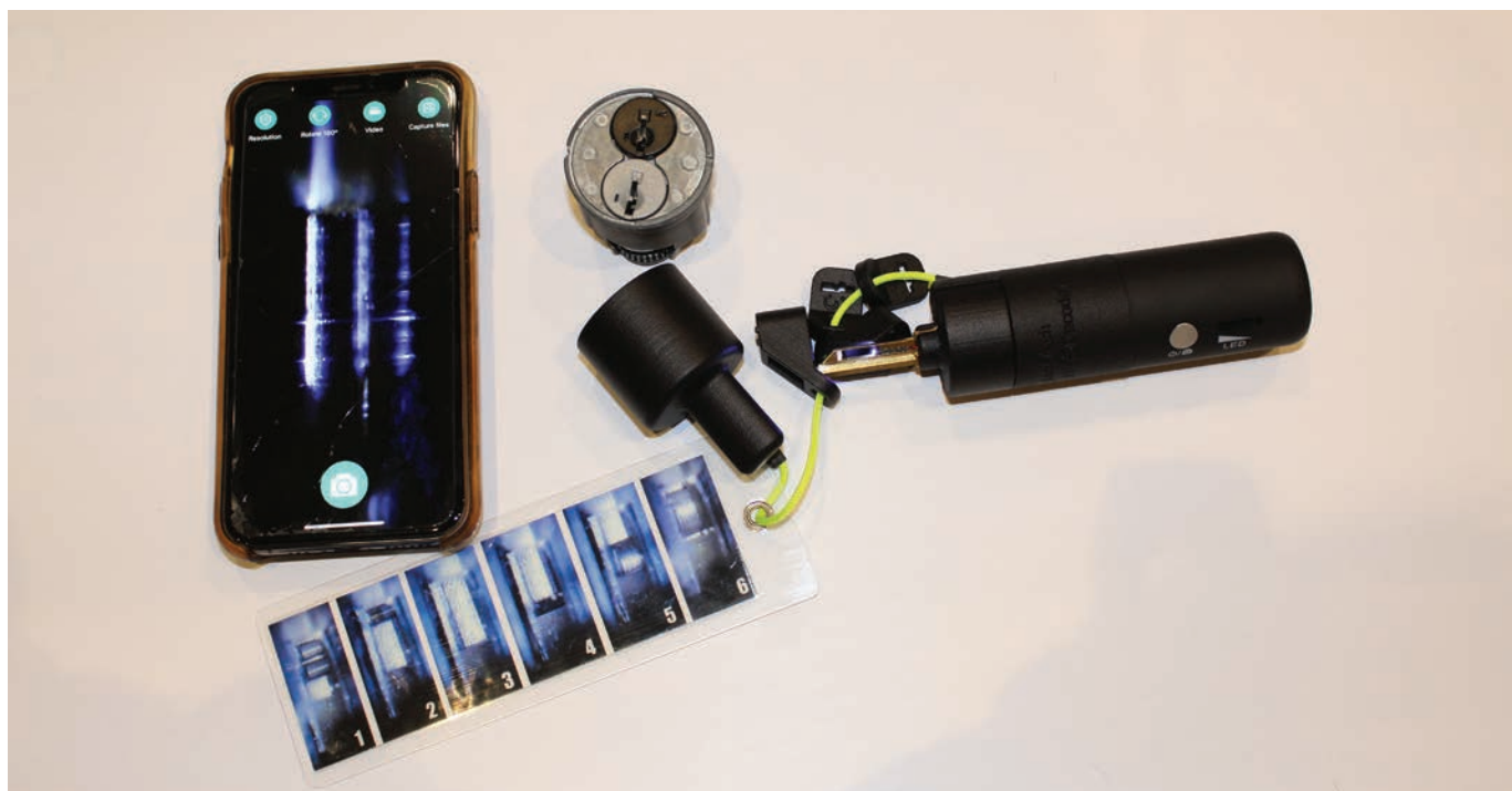
Figure 39. LockTech is a relatively new tool for decoding Kwikset Smartkey locks. The included chart makes it easy to determine the depth of the cut in each location. It comes with spacers to precisely place the camera at the correct location, or once you get used to the tool you can move the camera in or out without the spacers. The learning curve is very quick. Once the lock is decoded, simply cut a key to open the lock. If you run residential lockouts with Smartkey locks, you need this tool. Accureader.com is the company's website.
