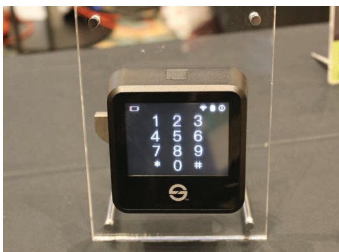
Figure 16. TimeMaster brought a few electronic safe lock keypads. The first one from S&G is a new touch screen keypad. It will retrofit to the Titan, 1004 and even the 6120.
