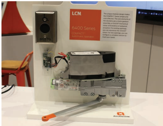
Figure 10. Allegion offers some great hardware and is always innovating. This year is no different. The LCN team has mated a motor assembly to the 4040 door closer. It mounts to all three mounting positions: top jamb and regular and parallel arm. It's designed for interior applications and must have a power supply and a couple of hardwired or wireless buttons to operate it. Best of all, it is a very simple retrofit to the basic closer, so it can be installed on new and existing doors. Allegion/LCN products are available at all the major distributors, or find info at us.allegion.com .
