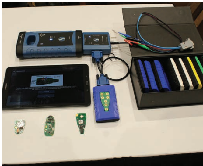
Figure 25. SmartBox offers a great programmer. The new model offers an optional adaptor to unlock remotes. You can use the probes or purchase the optional cradles to make it even easier, all at a very reasonable price. They can be found at smartboxauto.com.
