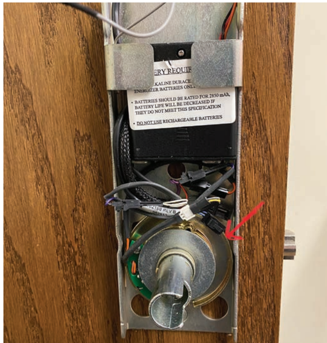
Figure 9. The arrow points to the inside ring through which the mounting screws, not visible here, attach to the cylindrical chassis.
