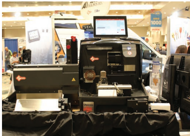
Figure 19. Ilco and Silca have a new key machine for high-volume cutters. The Unocode F900 is a variation of the Futura line that will auto load the blank from a stack of blanks, cut it and engrave it. These machines are in the $40,000 range, but if you are cutting a large batch of keys by code, this is the machine for you. You can find out more from your distributor or at dormakaba.com .
