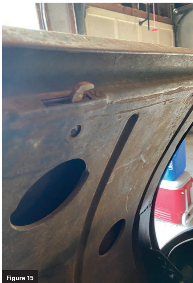
Figures 14-16. You can see the trunk lock handle, the hook bolt on the inside of the trunk and what it hooked into.
