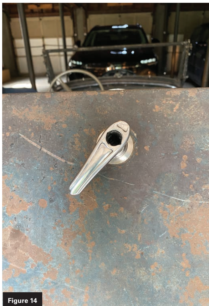
Figures 14-16. You can see the trunk lock handle, the hook bolt on the inside of the trunk and what it hooked into.
