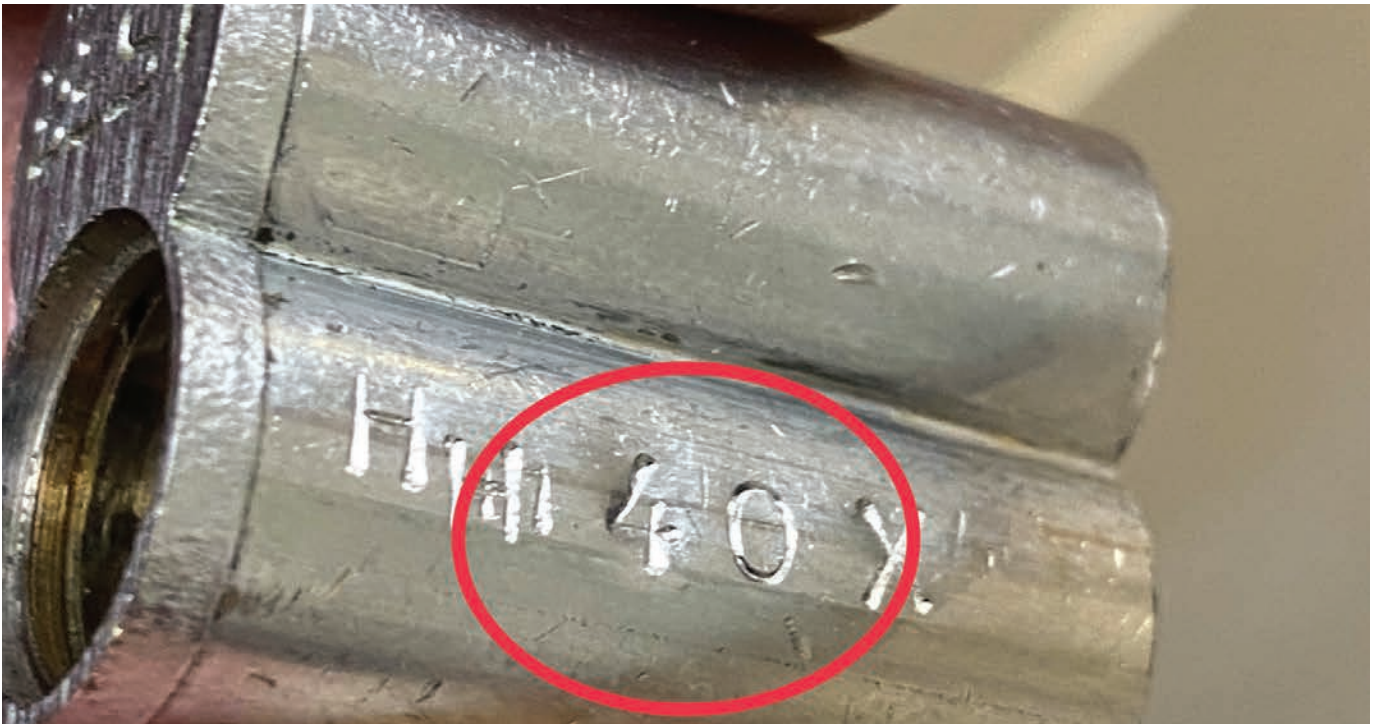
Figure 12. The author stamped the "top" part of the core that was actually the bottom, containing the plug.
