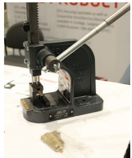
Figure 13. KSP is known for the great cylinders it produces. This year, the company designed and introduced the CPM-SFIC-150 small format IC capping press and strips. The strips enter in the side of the capping block and sit at an angle to make the caps punch one at a time as you move the punch down. It is an upgrade to the now-discontinued A-1 capping press, but if you have one, their strips will work in the old press. KSP is available at most major distributors or iccore.com .
