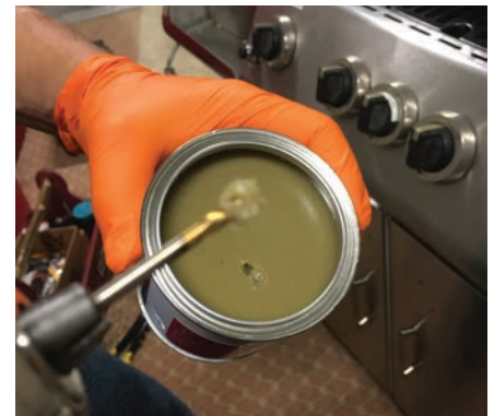
Figure 12. The author used a cutting paste called CUT-IT on his drill bits to help cut through the stainless steel.
