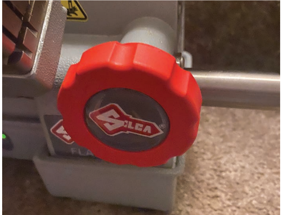
Figure 7. This image shows the red wheel that you turn to move the carriage and cut the key.
