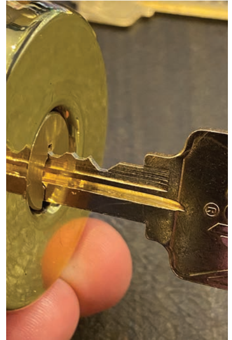
Figure 21. The newly cut key is partially inserted.
