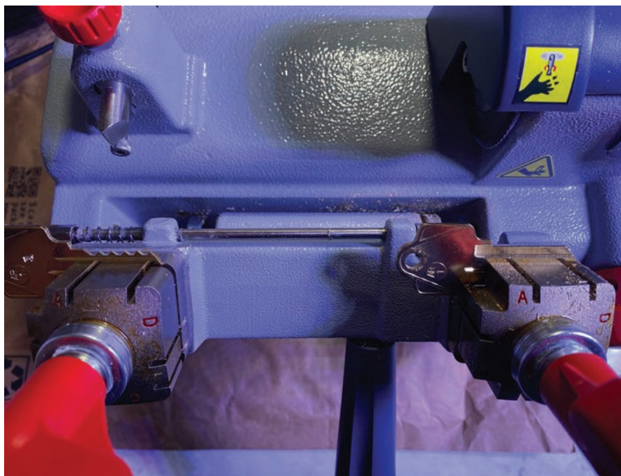
Figure 11. The number 3 depth key and blank are in the machine.
