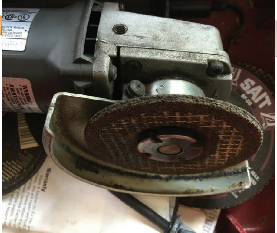
Figure 15. The author measured and cut the pieces of expanded metal with a metal cut-off wheel fastened to his 4 1/2" angle grinder.
