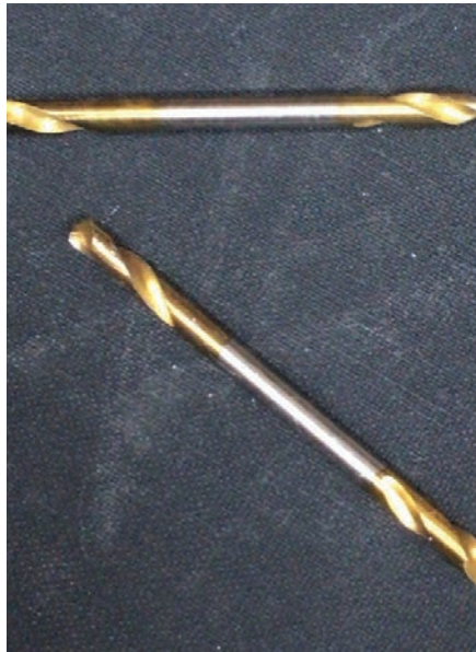
Figure 9. For this project, \frac{1}{8} " titanium high-speed double-end drill bits were used.
