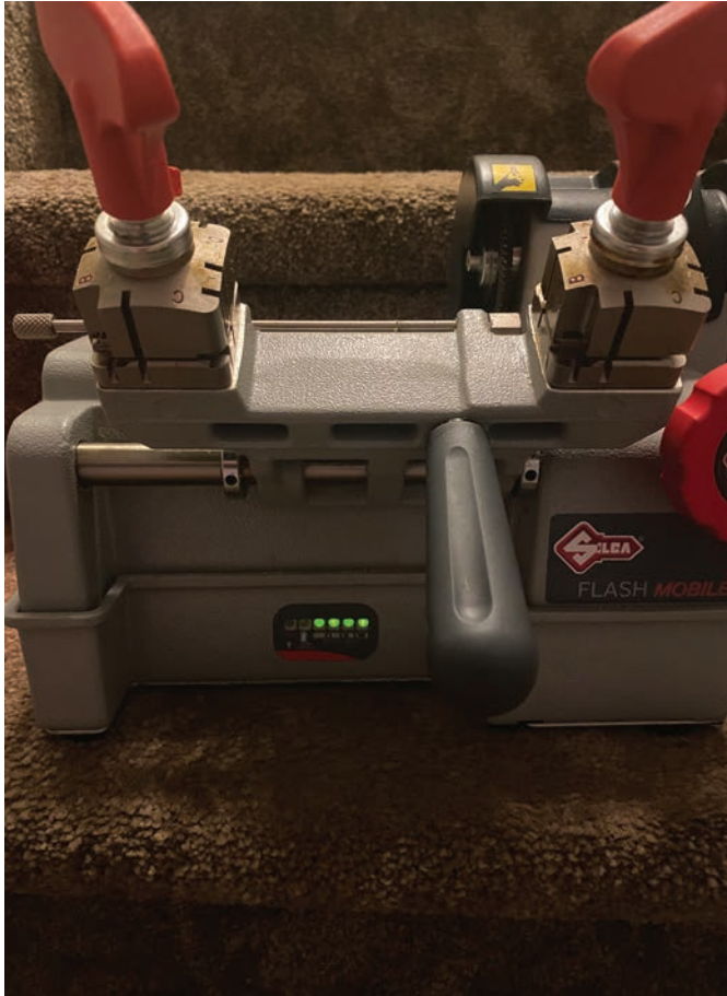
Figure 4. The power meter on the front of the machine lights up when the power button is depressed.
