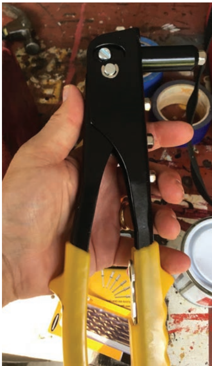
Figure 16. The author used a pop rivet tool to install a 3/16" x 1/4" fender washer under the head of each pop rivet.
