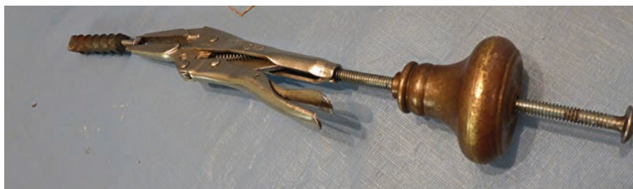
Figure 6. Using a homemade spline key puller, the author was able to pull two rebar plugs left by a previous tech.
