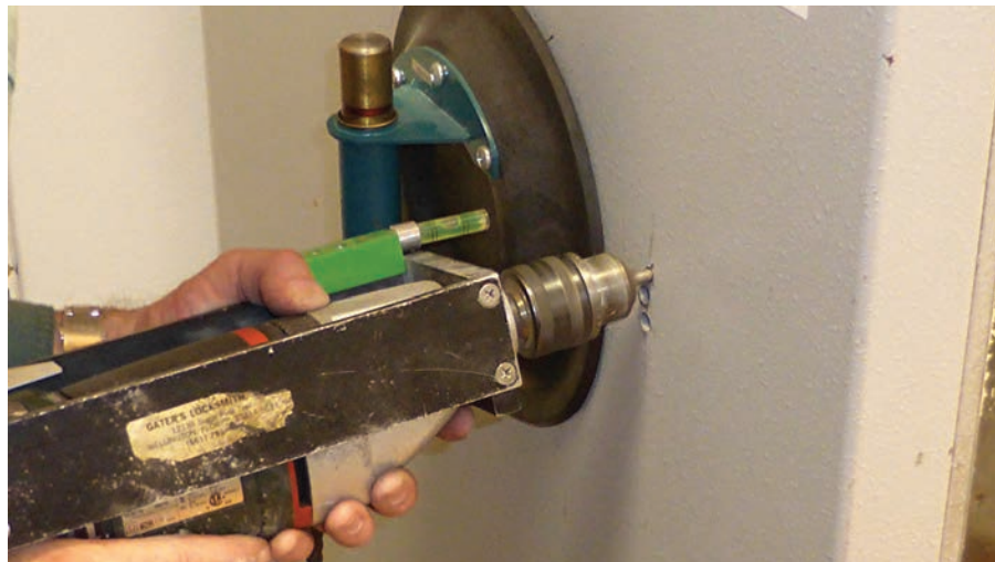
Figure 4. A suction cup was used to anchor the StrongArm lever rig and make drilling easier. The author used the hammer mode of the drill to get through the concrete body. In this photo, the author is drilling his third hole for inserting a scope to view the CKH. The first two holes hit the door locking bolt. The leveling tool on the rig was purchased from TimeMaster, Inc.
