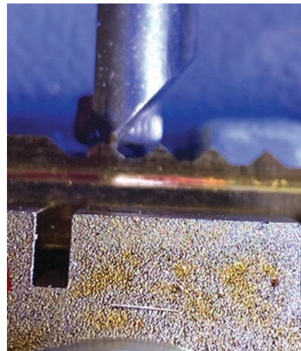
Figure 23. The stylus at the bow side of the depth key.
