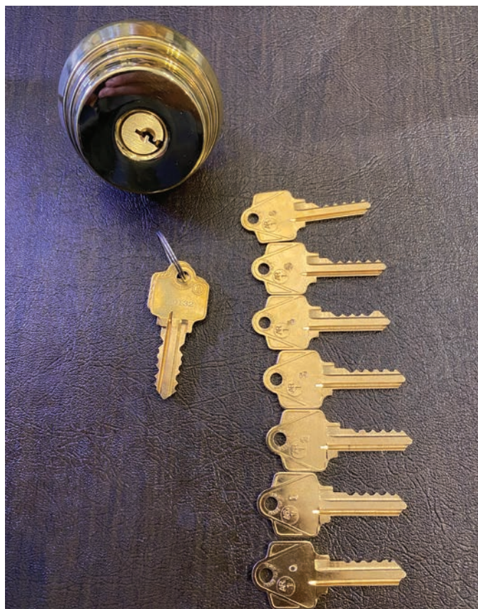
Figure 8. Here you can see a deadbolt, a pair of original keys with the bitting numbers (30132) stamped on them, and seven Arrow depth keys from 0 to 6.
