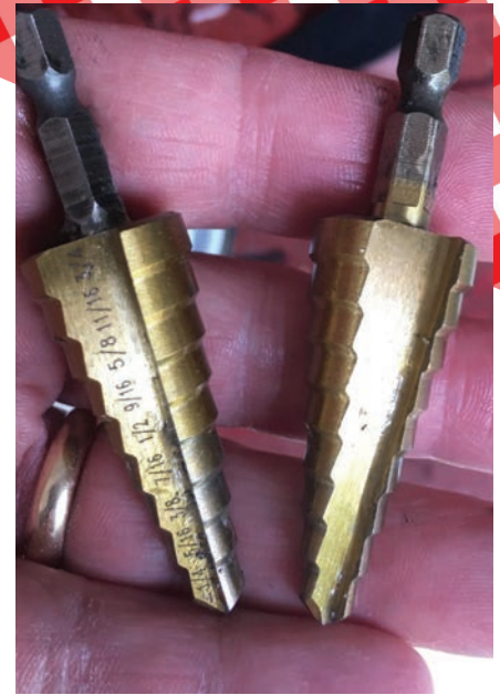
Figure 11. The holes were finished with a titanium nitride step bit.
