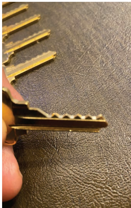
Figure 10. The key has a code of 66666.
