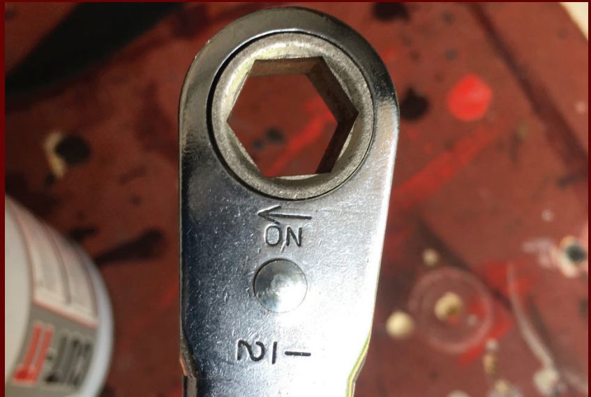
Figure 19. Use a ratcheting wrench to speed the installation of carriage bolts, lock washers and nuts.
