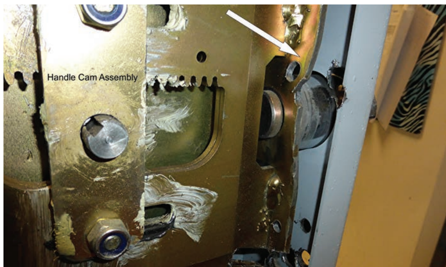
Figure 9. The author's desperate attempt to punch the bolts back only succeeded in bending the carrier bar (and potentially much worse). Marking the BCH showed there was no progress even though the punch moved deeper with each whack of the hand sledge. The author came to his senses and aborted the procedure.
