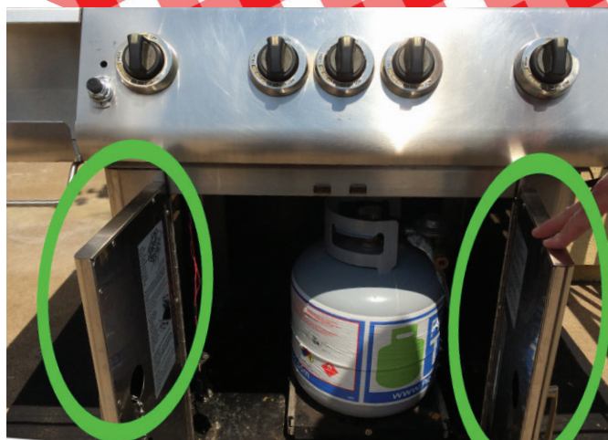
Figure 2. The grills had double doors made from two sheets of stainless steel.
