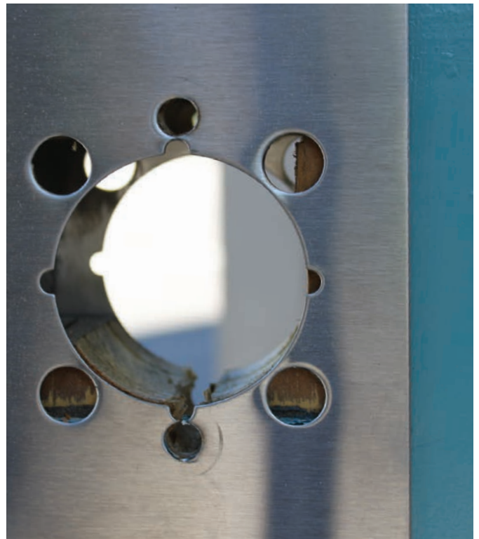
Figure 8. We used the plate to guide a hole saw to open the cross bore and drill the two through-bolt holes.
