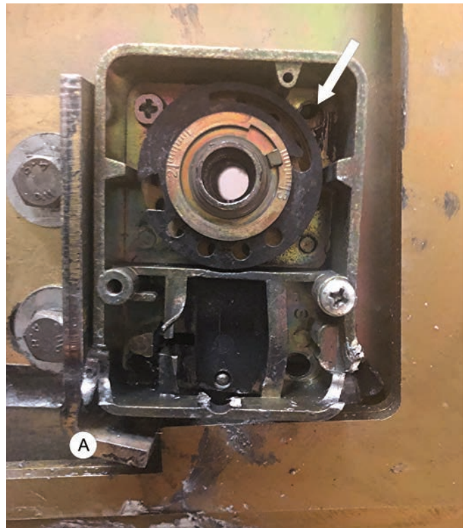
Figure 2. This photo was taken immediately after the door was opened. The arrow shows where the mounting screw would have fallen and wedged between the wheels and lock case. Notice the bottom two mounting screws are missing as well. A little thread locker could have prevented this lockout. The author was told this safe was serviced just six months before this malfunction.
