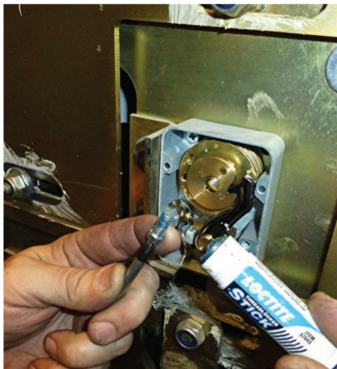
Figure 15. Immediately after opening the safe, the author applied Loctite to all four mounting screws in the remaining lock.
