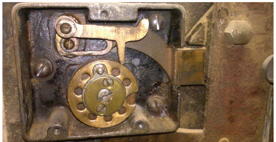
Figure 13. The nose is riding on top of the wheels.
