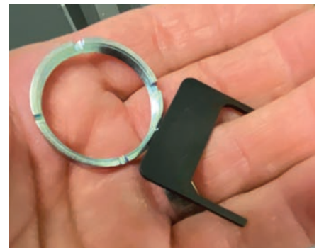
Figure 7. The cylinder nut and the tool for tightening it were stashed in the cylinder hole.
