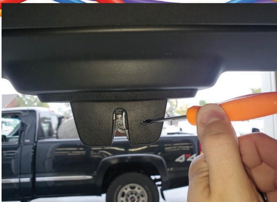
Figure 10. Push toward the latch with the small screwdriver to release the trunk latch.
