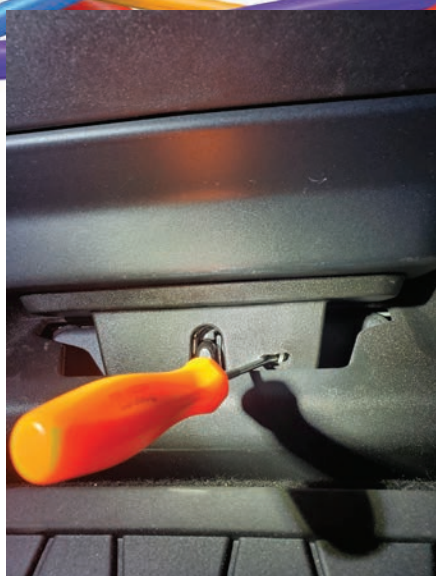
Figure 9. The hole next to the emergency trunk latch will allow you to manually move the latch with a poker or small screwdriver.
