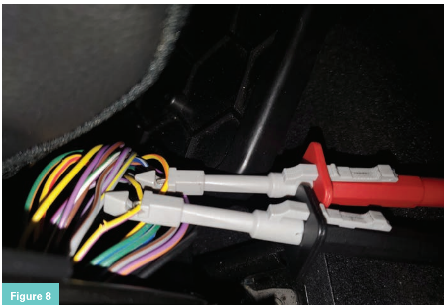
Figures 7 and 8. The probes are connected to the yellow/orange and yellow/purple wiring under the driver's seat.
