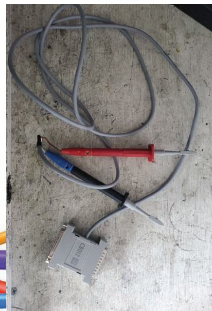
Figure 2. The author used these cables with Arites to connect into the CAN bus lines.
