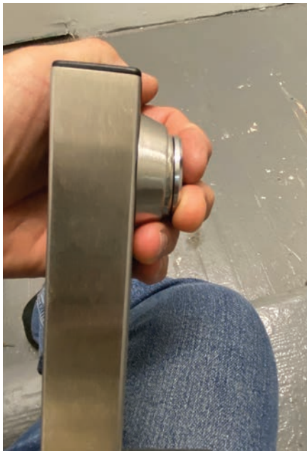
Figure 10. This image shows the rings the author used to get the cam to hit where it needed to.
