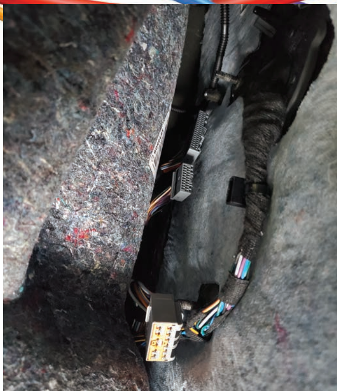
Figure 14. The module has three plugs on the underside that are somewhat difficult to remove due to limited space.
