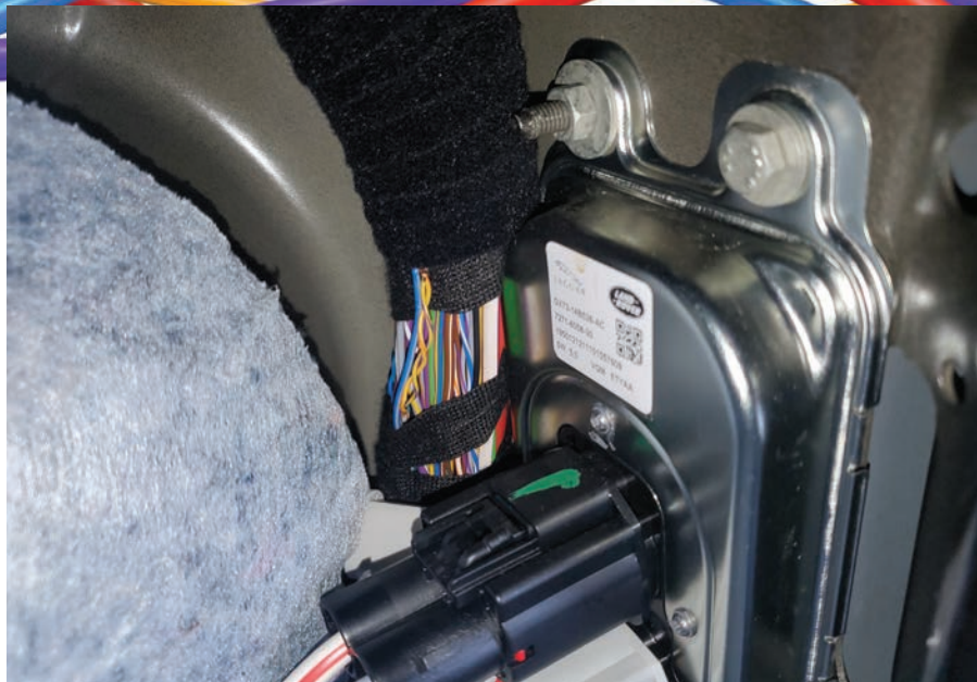
Figure 17. This shows the location of the CAN bus wires in the passenger-side trunk compartment, close to the taillight.
