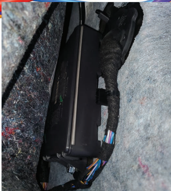
Figure 13. There are plastic clips to hold the wiring harness in place on the bolts that the KVM attaches to. One was under the 10 mm nut, and the other was on top, preventing removal of the nut.
