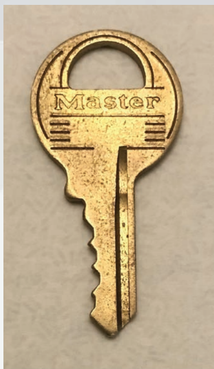
Figure 24. The author originated the key using a HPC 1200CM code machine with the key cuts 3453 on an original Master 1K key blank.
