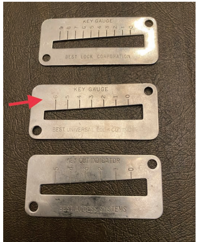
Figure 2. The arrow points to the number 6 depth on the A3 gauge.
