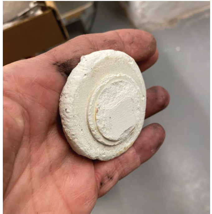
Figure 18. The author knocked off the plaster disk by putting the blade of a putty knife against it and tapping.
